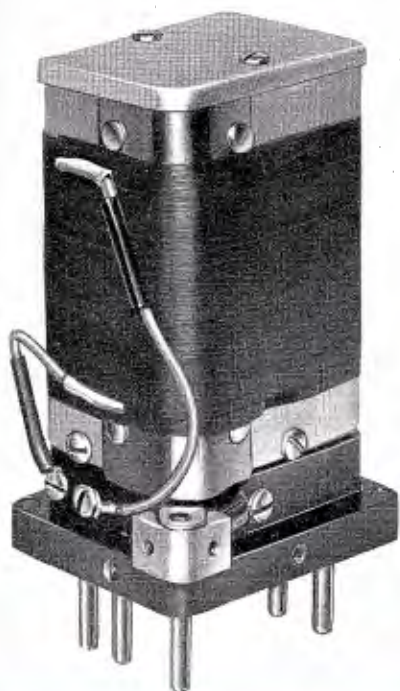
A TMV-129 type Crystal Unit with outer case removed to show 14-watt heater and mounting base.
